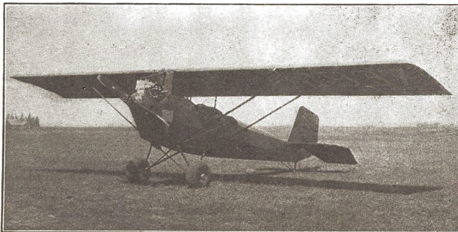
This Pietenpol Air-Camper is one for you birds who want to buy 'em knocked down. B. H. Pietenpol, of Spring Valley, Minn., makes them. The price complete is $850, or as we have just said, you may buy the parts and assemble the job yourself. With the converted Ford Model "A" engine, the top speed is 90 m.p.h. The cruising range is 230 miles.
